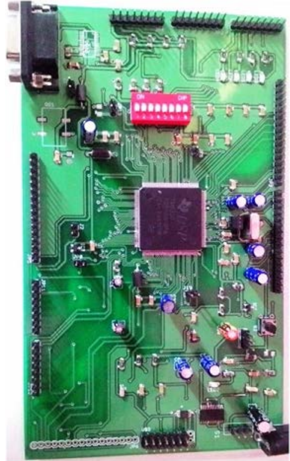
Fig. 11: Finalized DSP Board
